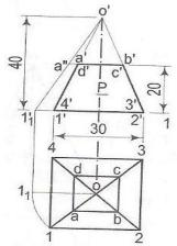
6: Draw the development of the lateral surface of the truncated cone as shown in the figure.
