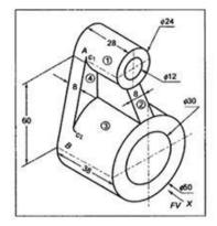
2: Orthographic projection – Draw the Orthographic Projections of the object given below in 1<sup>st</sup> angle method of projection. (1) Front View (2) Top View (3) R.H.S.V.
