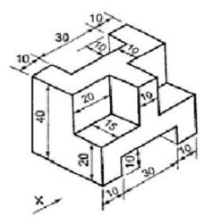
3: Figure shows isometric projection of an object. Draw the following views: (1) Front View(2) Top View (3) Side View by first angle projection Method.
